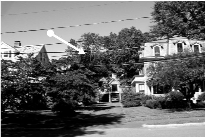
Low-hanging wires tied (at center of photo) to keep trucks from knocking them down. (Photos by Lois Beiner)
