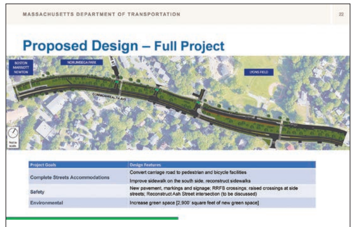
Commonwealth Ave Carriageway Full design. Graphic image of the Commonwealth Ave Carriageway between Lyons Field and Auburn St. where it will merge with the replaced Rt 30. Charles River Bridge. Courtesy Ted Chapman
