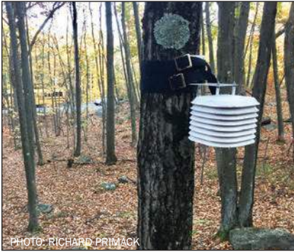
Air temperature monitor on a tree.
