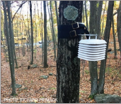
Air temperature monitor on a tree.
